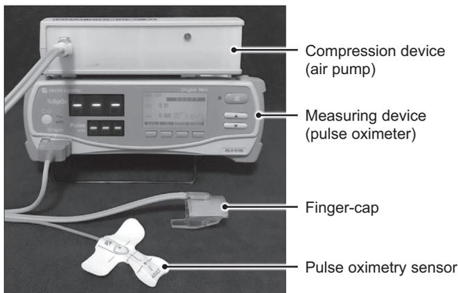
Fig. 1. The investigation device is composed of two devices, which are modified pulse oximeter (measuring device) and compression device. A pulse oximetry sensor is attached to the measuring device and the compression device controls a bladder cuff inside a finger-cap.
