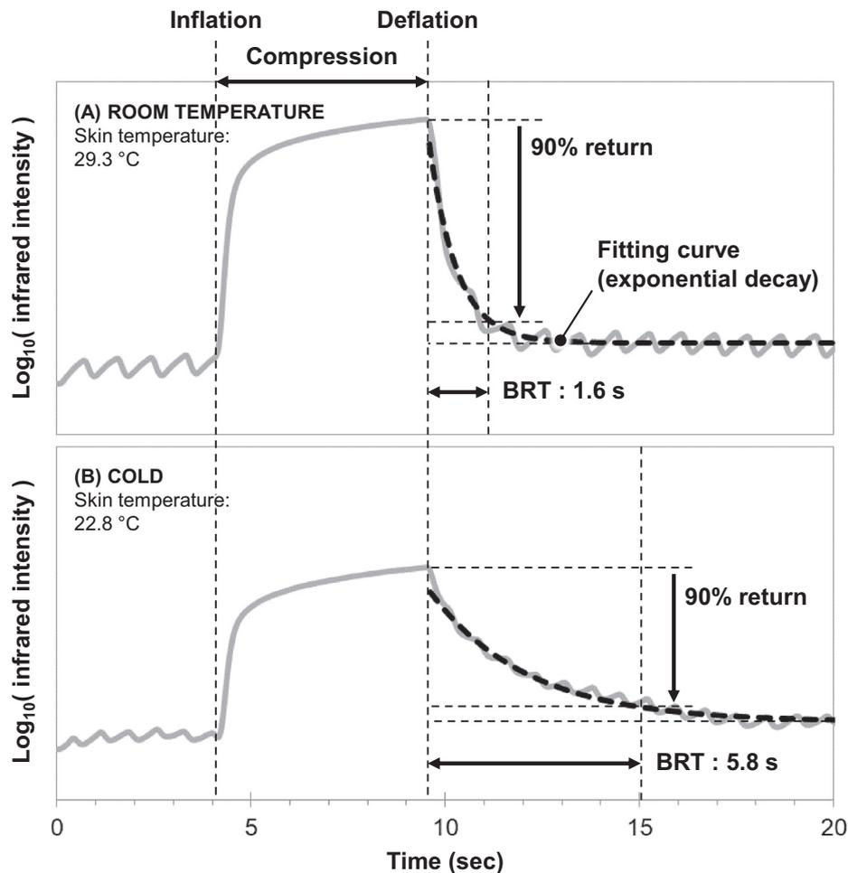
**Fig. 3.** The measuring device captures the changes in the transmitted light intensity and records the waveforms. The time to achieve 90% return of the intensity was reported as BRT. BRT was measured at two different temperature conditions of a healthy subject.
